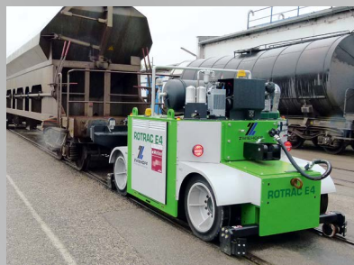
ROTRAC E4 Shunting capacity up to 500 t
