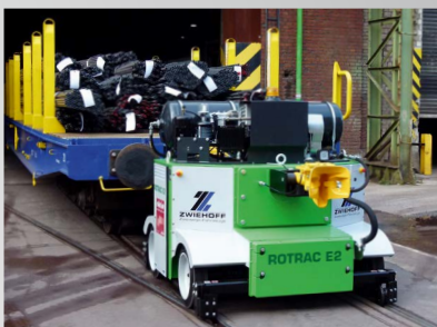
ROTRAC E2 Shunting capacity up to 250 t
